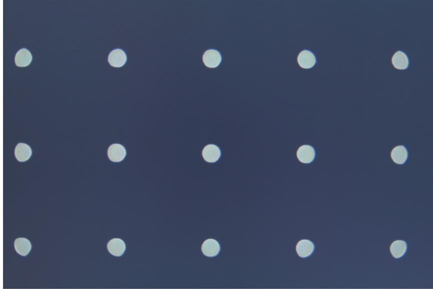
Figure 1.2: Defocus PSF acquired by deliberately defocusing an LCD covered by regularly spaced white dots. Vignetting clips the polygonal shape of the PSF, especially on the periphery of the field of view.
